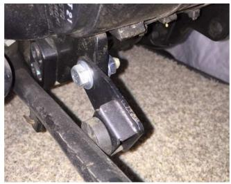
Align stop bracket and kickstand and complete final tightening. You can affect the kick stand distance from the muffler by rotating the kickstand stop bracket clockwise/counterclockwise.
