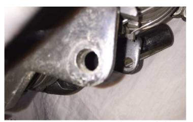
This is the frame tab that you will attached the bracket to. It is on the left side "ear" on lower frame under engine. It would be where centerstand would normally bolt.
